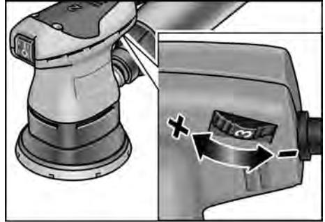
The thumb wheel can be used to steplessly vary the number of oscillations from 1 (low) to 6 (high) even while the power tool is running.
