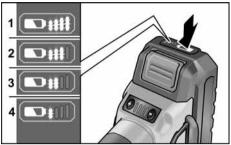
The indicator goes out after 5 seconds. If one of the LEDs flashes, the battery must be recharged. If none of the LEDs light up after the button is pressed, the battery is faulty and must be replaced.
