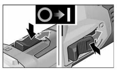
To switch off the power tool, release the switch rocker by pressing the rear end.
