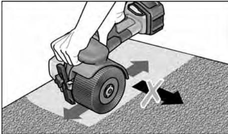
Place the power tool carefully on the surface to be treated and guide it back and forth with linear movements.
