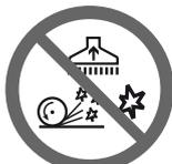
Do not extract glowing dust or other ignition sources. Do not use in conjunction with machines that generate sparks!
