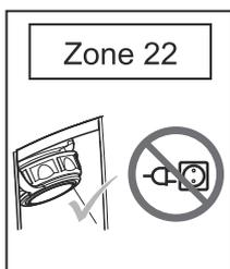
Keep the socket on the appliance closed in zone 22. Do not use the socket on the appliance in zone 22.
